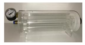
The tester consists of one or more interchangeable clamp shelf units and a minimum size vacuum container. The clamp shelf unit with integrated lid and handle is tightly fitting in the fully (360°) transparent vacuum container.
