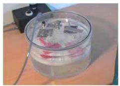
A grid integrated in the lid and a floating plate in the bowl hold the samples in fixed positions throughout the test. The Water Vacuum Bowl is equipped with a pneumatic vacuum pump, capable of obtaining -80% vacuum in less than 20 seconds.
