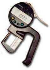
Owing to the self-adjusting measuring force, the Thickness Gauge can be used in various positions with retained accuracy. For instance, the gauging can be done on specimen mounted in a tensile testing machine.
